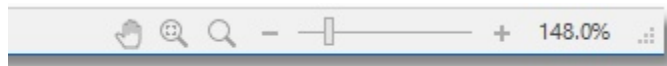
Figure 3-23: View tools: Auto Pan, Zoom to Fit, Zoom Rectangle, slider bar, zoom percentage
